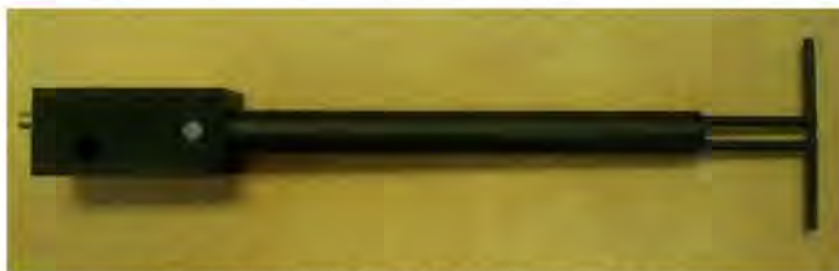
Figure 1 – MVG COMOSAR Validation Dipole
