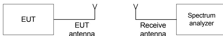
Figure 7.3.1 Occupied bandwidth test setup
