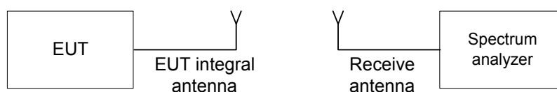
Figure 7.1.1 Setup for transmitter shut down test
