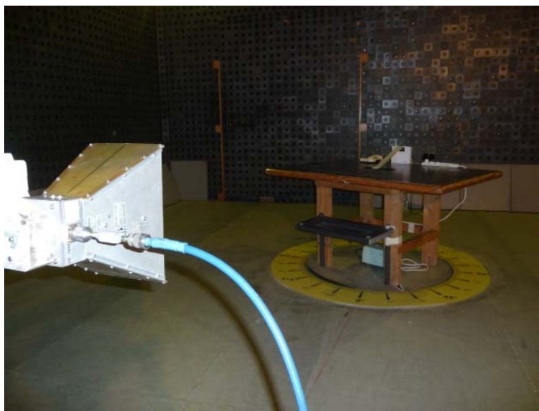
Photograph 8.2.2 Setup for spurious emission field strength measurements above 1000 MHz
