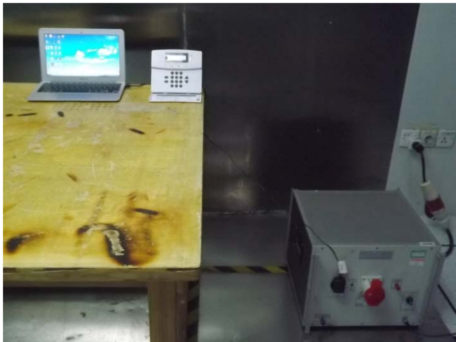
Conducted Disturbance at Mains Terminal Test Setup
