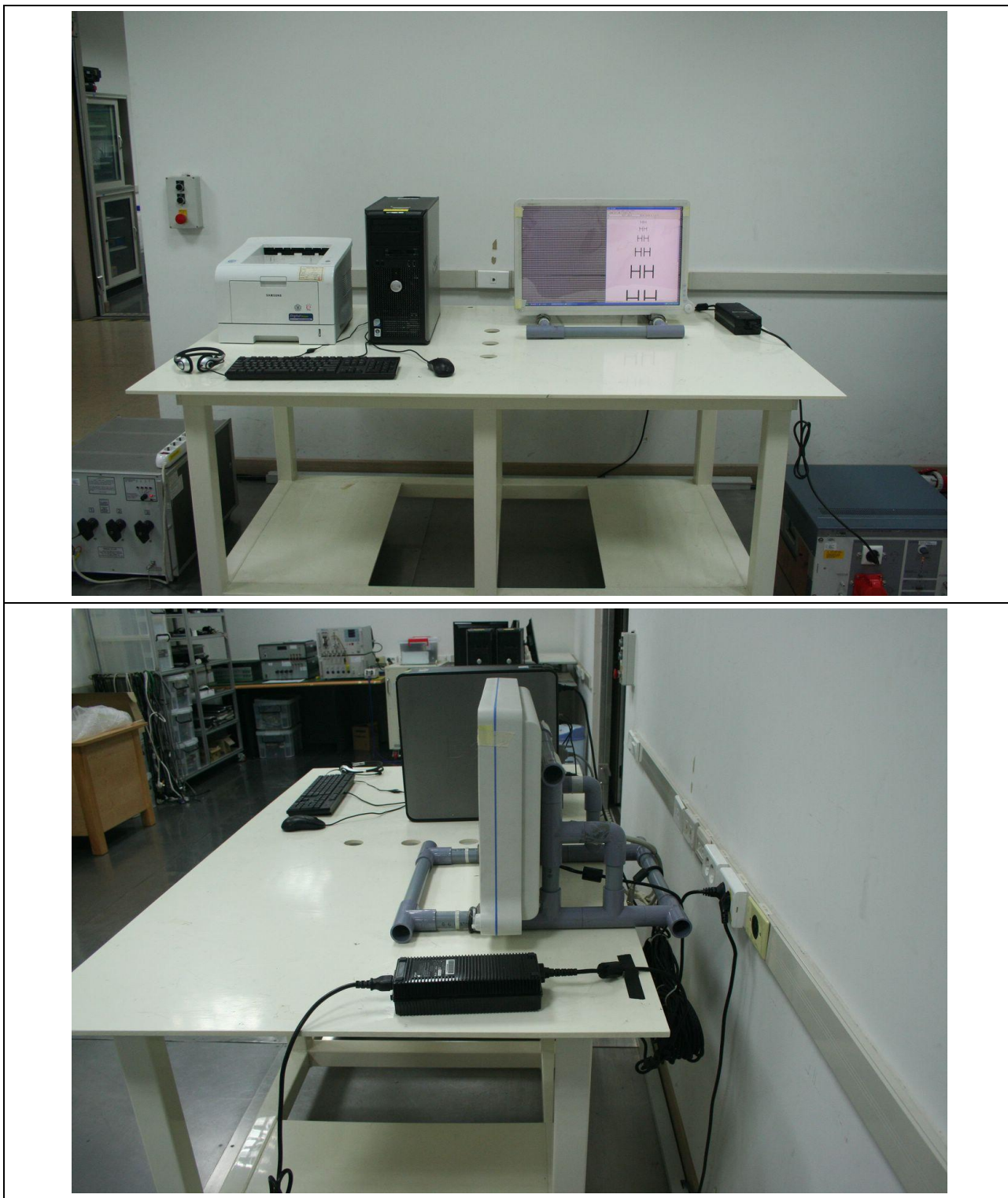
Figure 1. Conducted Emission Test Setup for DVI Mode:
