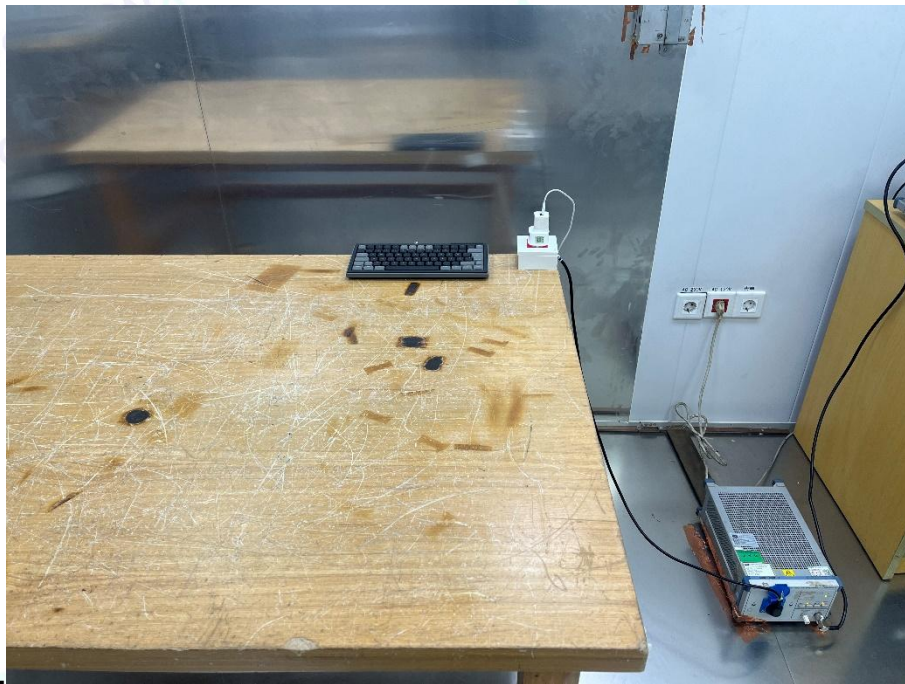
Photo of Setup for Radiated Emission (30MHz~1GHz)
