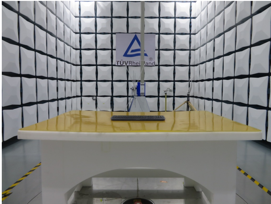
Photograph 2: Set-up for Radiated Spurious Emission, above 1GHz
