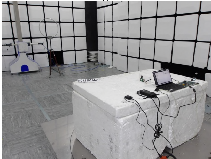
Photo 1.5-2 – Back View of the Test Setup, 3m - Out of band emissions below 30MHz
