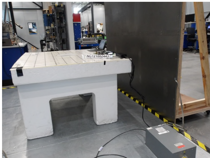
Photo 1.2-2 – Conducted Emission Test Setup [Front View]
