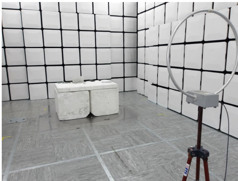
Photo 1.3-1 – Front View of the Test Setup, 3m - Operation within the band 13.110-14.010 MHz
