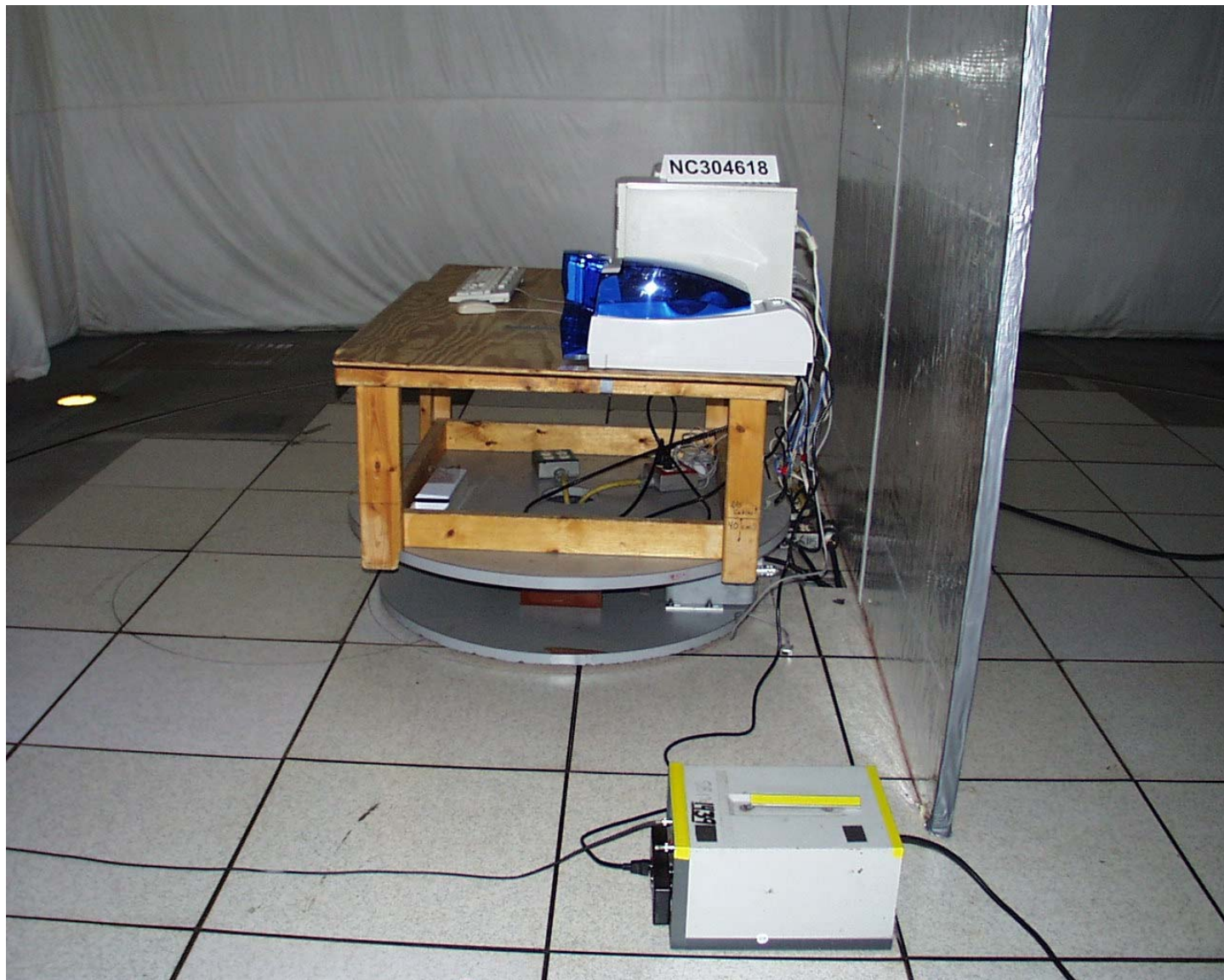
Test-setup photo(s): Conducted emission 150 kHz - 30 MHz
