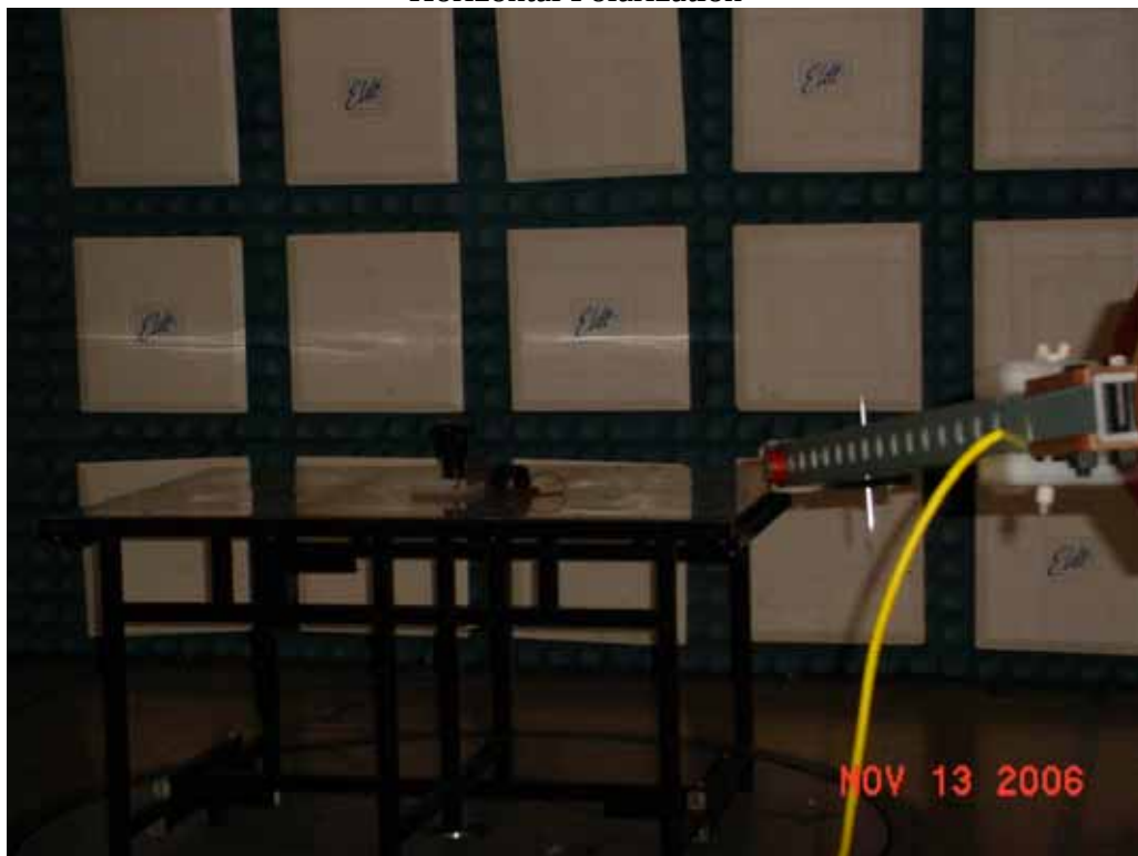
Test Setup for Radiated Emissions, 916.45MHz, with no metal enclosure – Vertical Polarization
