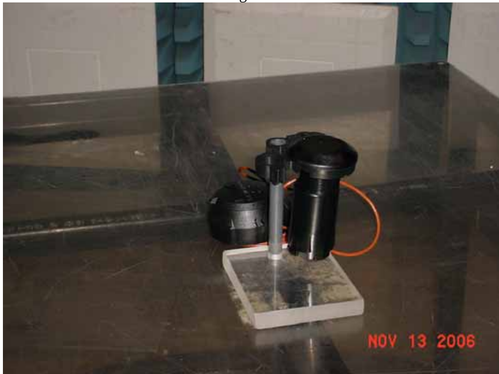
Test Item Setup, with no metal enclosure
