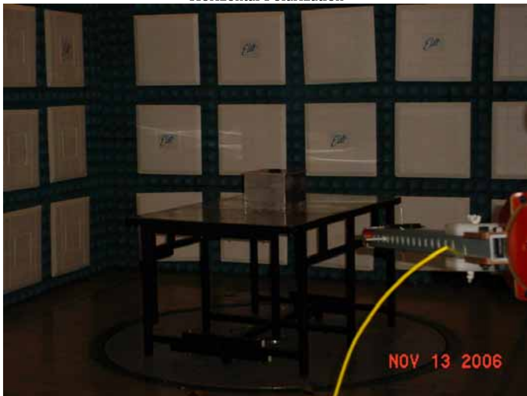
Test Setup for Radiated Emissions, 916.45MHz, with metal enclosure – Vertical Polarization
