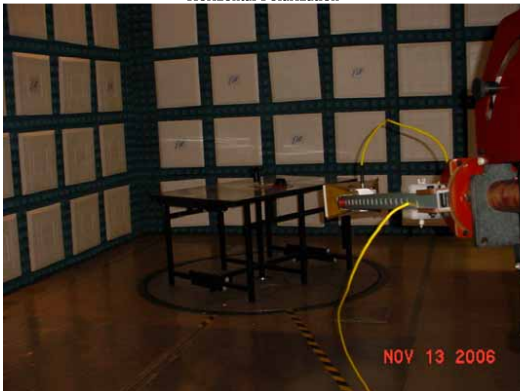
Test Setup for Radiated Emissions, 1GHz to 10GHz, with no metal enclosure – Vertical Polarization
