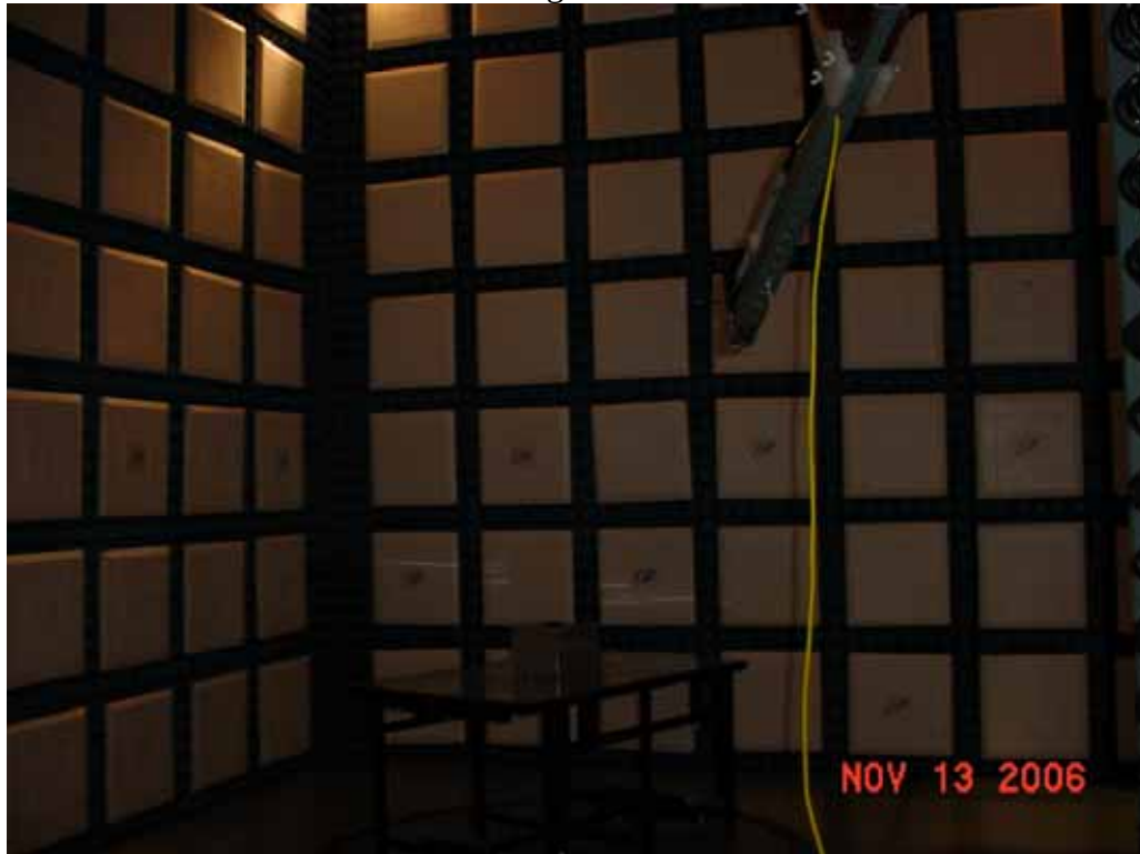
Test Setup for Radiated Emissions, 911.65MHz to 921.25MHz, with metal enclosure – Horizontal Polarization
