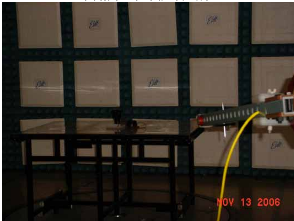
Test Setup for Radiated Emissions, 911.65MHz to 921.25MHz, with no metal enclosure – Vertical Polarization
