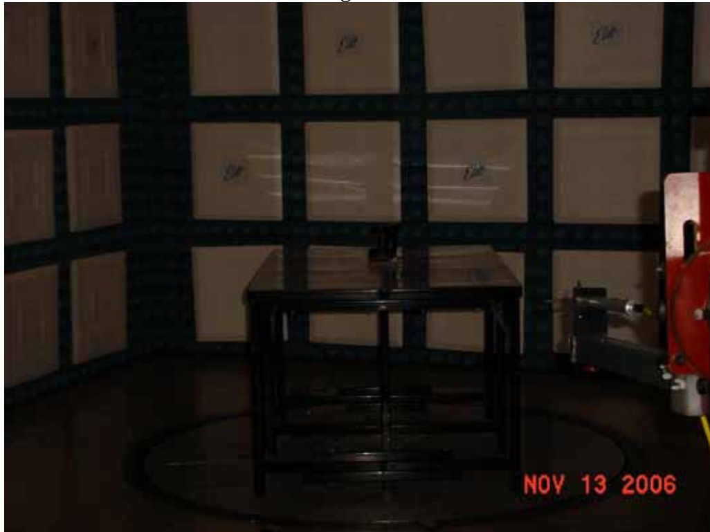
Test Setup for Radiated Emissions, 911.65MHz to 921.25MHz, with no metal enclosure – Horizontal Polarization
