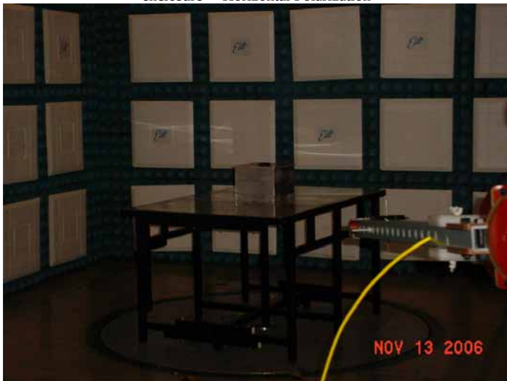
Test Setup for Radiated Emissions, 911.65MHz to 921.25MHz, with metal enclosure – Vertical Polarization
