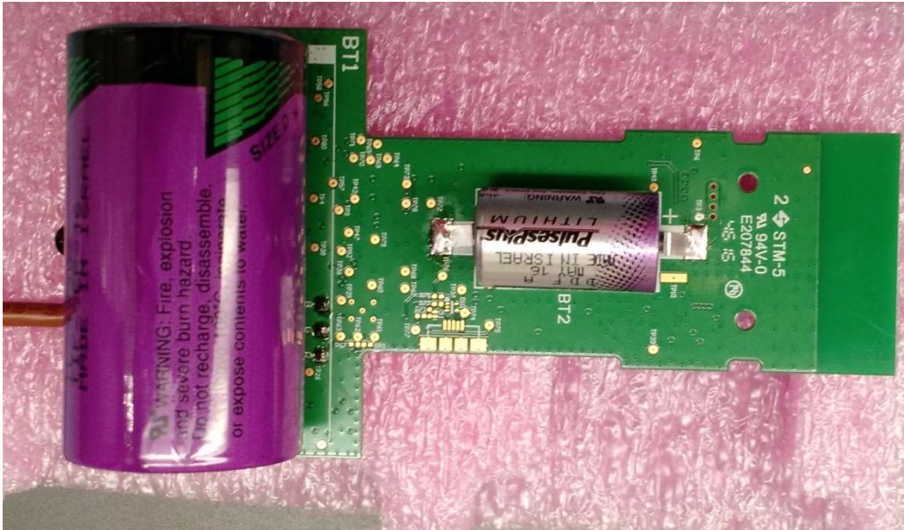
Figure 3 Batteries installed on PCBA.
