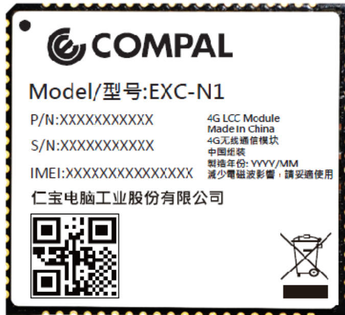
Figure 5-2 LCC Module Laser Marking
