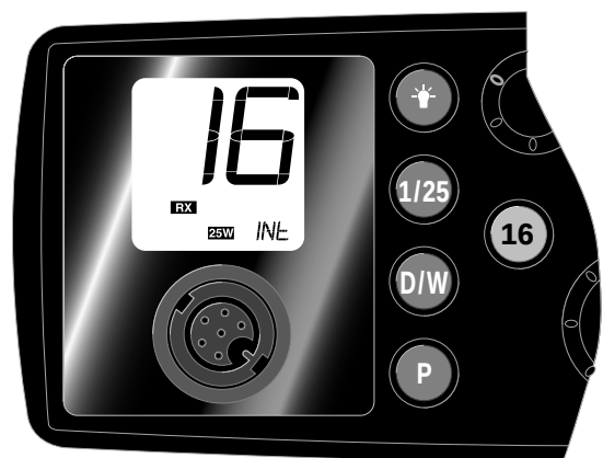
Fig 2.7 - Controls – non-scanning versions
