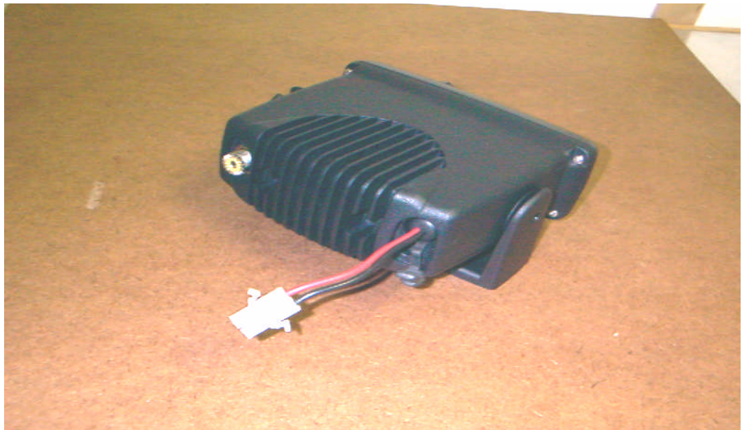
PHOTOGRAPH 11 Rear view of RD62 radiotelephone
