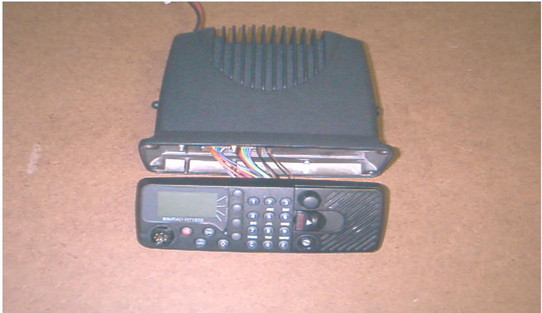
PHOTOGRAPH 12 RD62 showing the Rx/Tx & front panel sections
