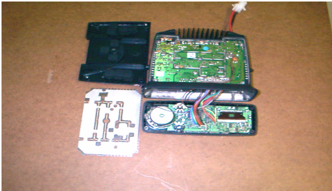
PHOTOGRAPH 13 Internal view of the Rx/Tx transceiver, front panel, screen & lid sections
