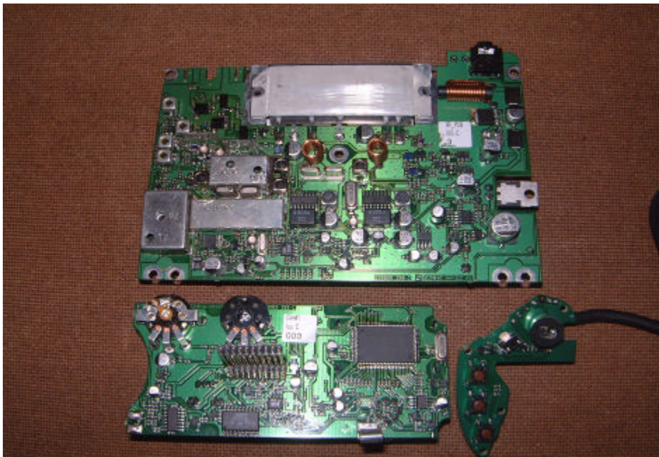
PHOTOGRAPH 6 RT63 Rx/Tx PCB & front panel PCB
