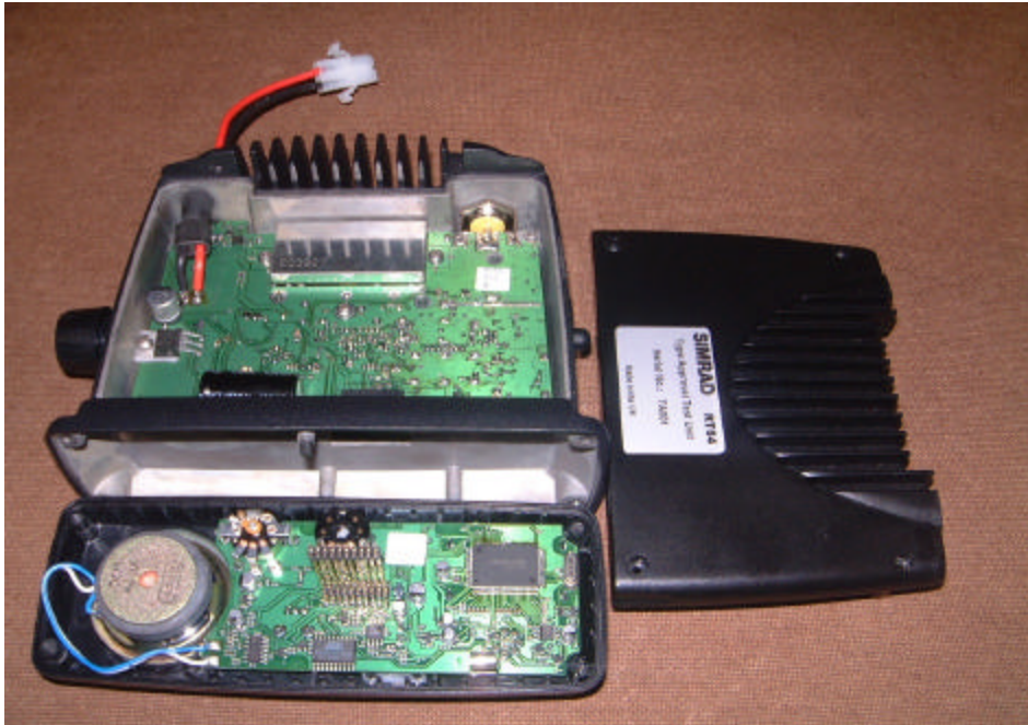
PHOTOGRAPH 5 RT63 showing the Rx/Tx & front panel sections
