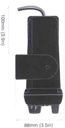
Fig 3.2 - Minimum clearance required
