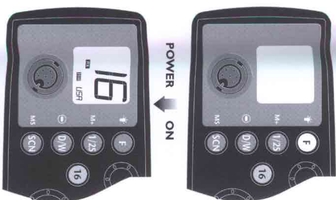
Fig 2.8 - Selecting secondary channel set
