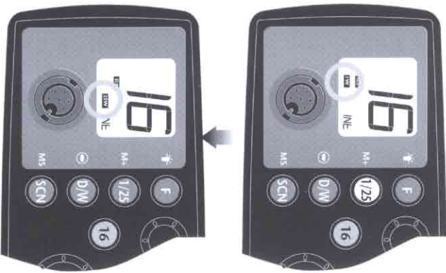
Fig 2.3 - Selecting transmission power (1/25W)
