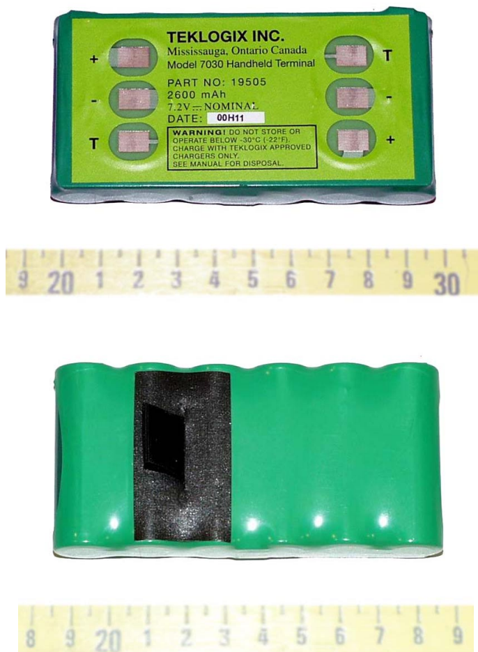
< Rechargeable battery P/N:19505, 7.2V/2600mAh >
