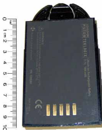
< Lithium-Ion rechargeable battery (M/N: F41001658, 11.1V, 1900mAh) >
