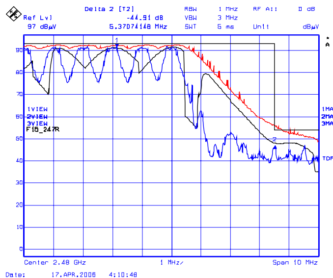
Plot 5.7.5.1.10 Band-Edge Radiated Emissions @ 3 meters, Vertical Polarization Upper End of Frequency Band (2480 MHz), Frequency Hopping Enabled
