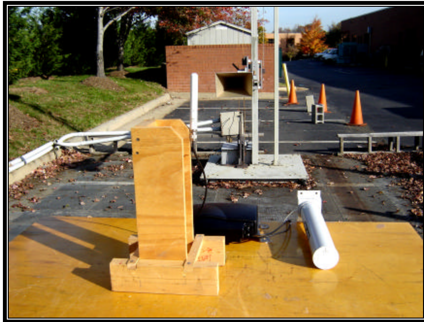
Photograph 17: Radiated Testing – 6 dBi Radiall Omni Rear View
