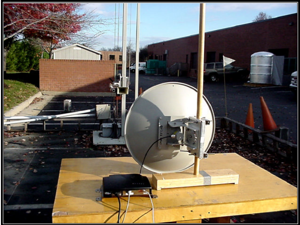
Photograph 9: Radiated Testing – 28 dBi Gabriel Dish Rear View
