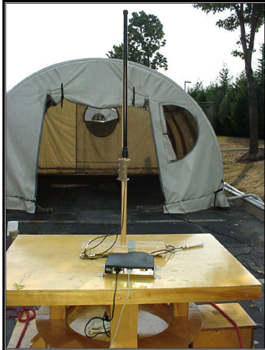
Photograph 4: Radiated Testing – 12 dBi Collinear Omni Front View
