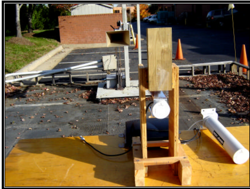
Photograph 14: Radiated Testing – 10 dBi MaxRad Panel Front View
