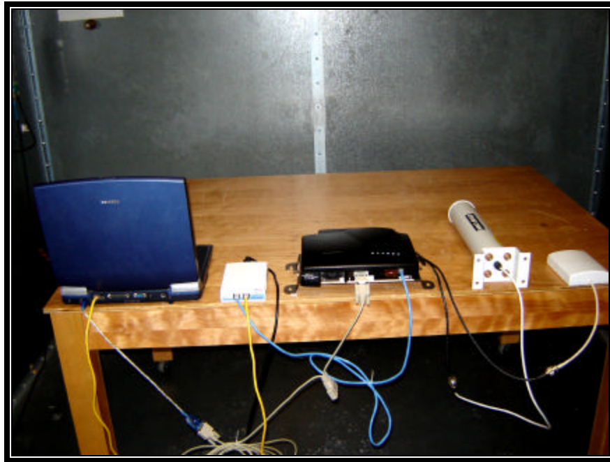
Photograph 21: Conducted Line Emissions Testing; Powered over Ethernet - Rear View
