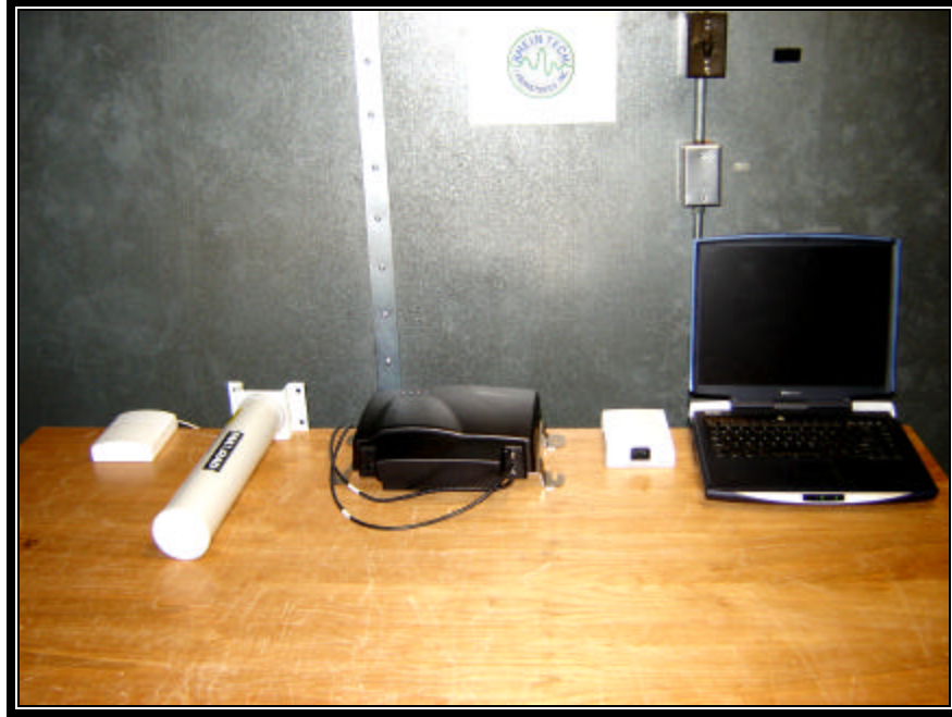
Photograph 18: Conducted Line Emissions Testing; AC Powered - Front View
