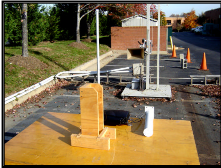
Photograph 11: Radiated Testing – 12 dBi Pacific Collinear Omni Rear View
