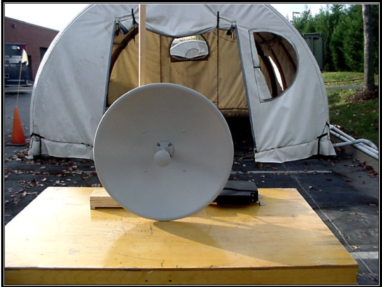
Photograph 8: Radiated Testing – 28 dBi Gabriel Dish Front View
