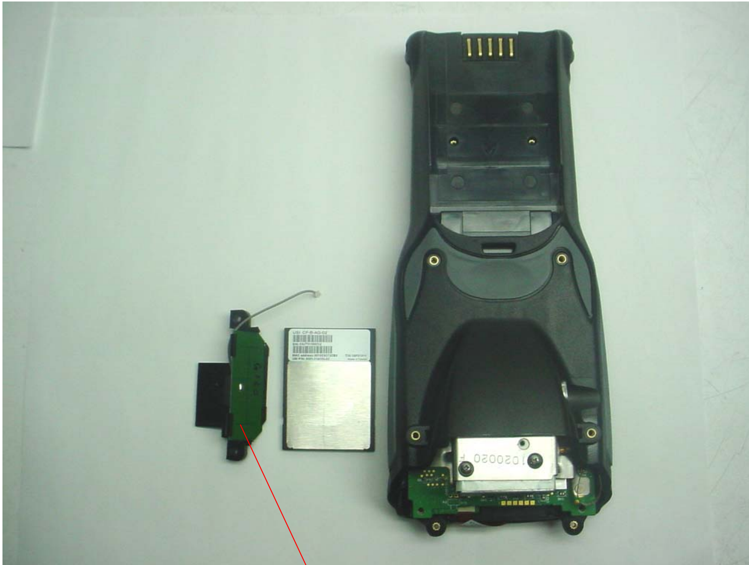
Psion Teklogix Antenna, Model: 1020096-100, Gain 0 dBi
