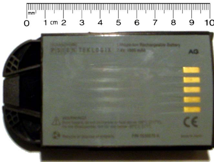
< Lithium-Ion rechargeable battery (P/N: 1030070 A-001, 7.4 V, 1800 mAh) >
