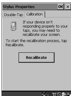
Figure 5.22 Calibrating The Touchscreen
