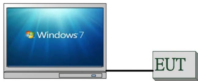
Fig. 2-2 Conducted (Antenna Port) Configuration
