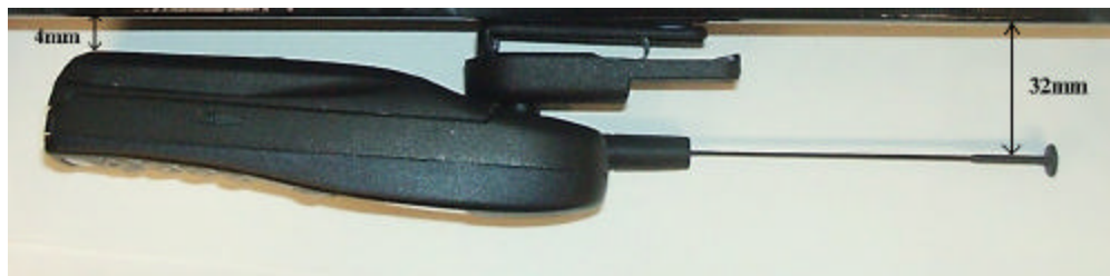
Picture 2. Separation distance with Belt Clip BCH-12U
