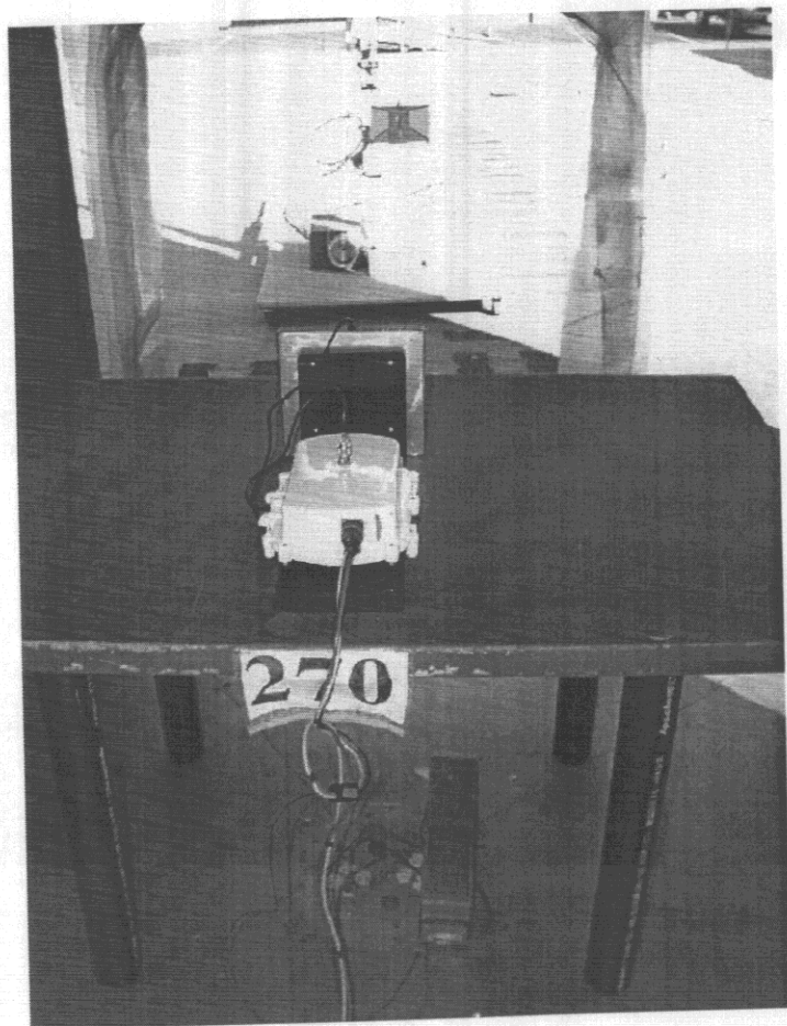
Radiated Emissions in Restricted Bands test setup
