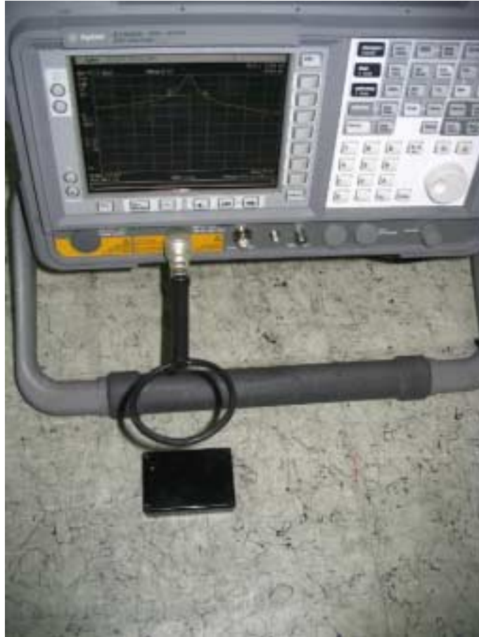
Photograph No.6 Setup for occupied bandwidth test
