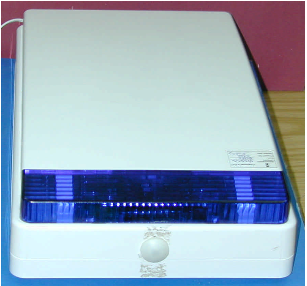
Photograph No.1 Wireless siren General view
