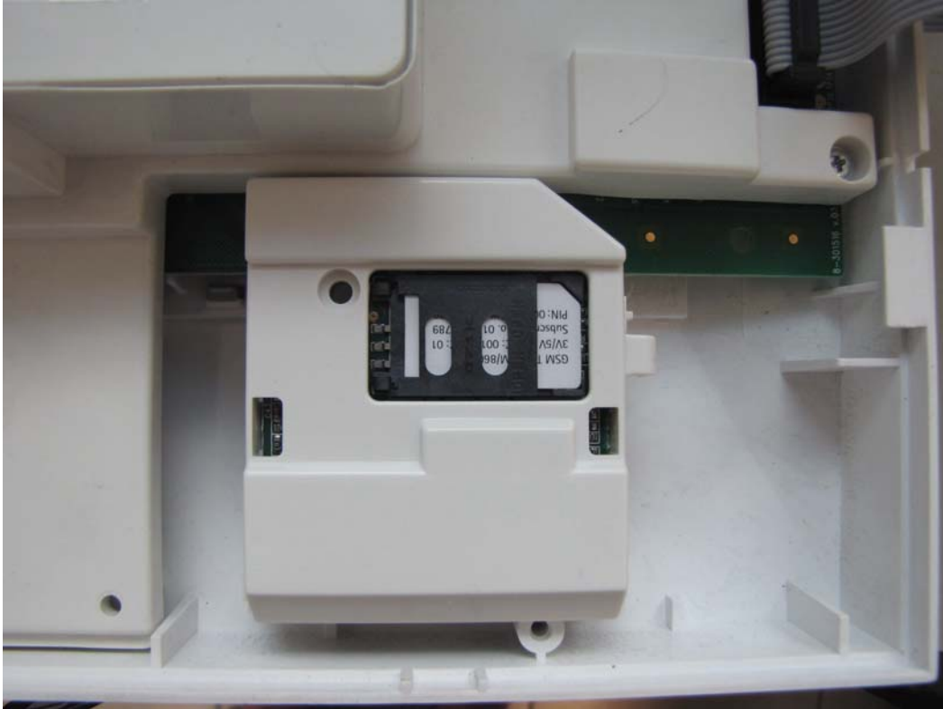
Photograph No.2 PowerMax Pro GSM modem view
