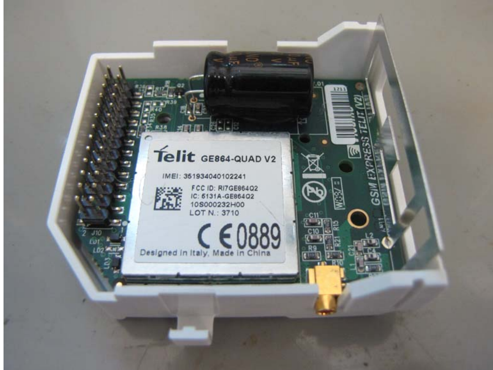
Photograph No.6 GSM modem rear side view
