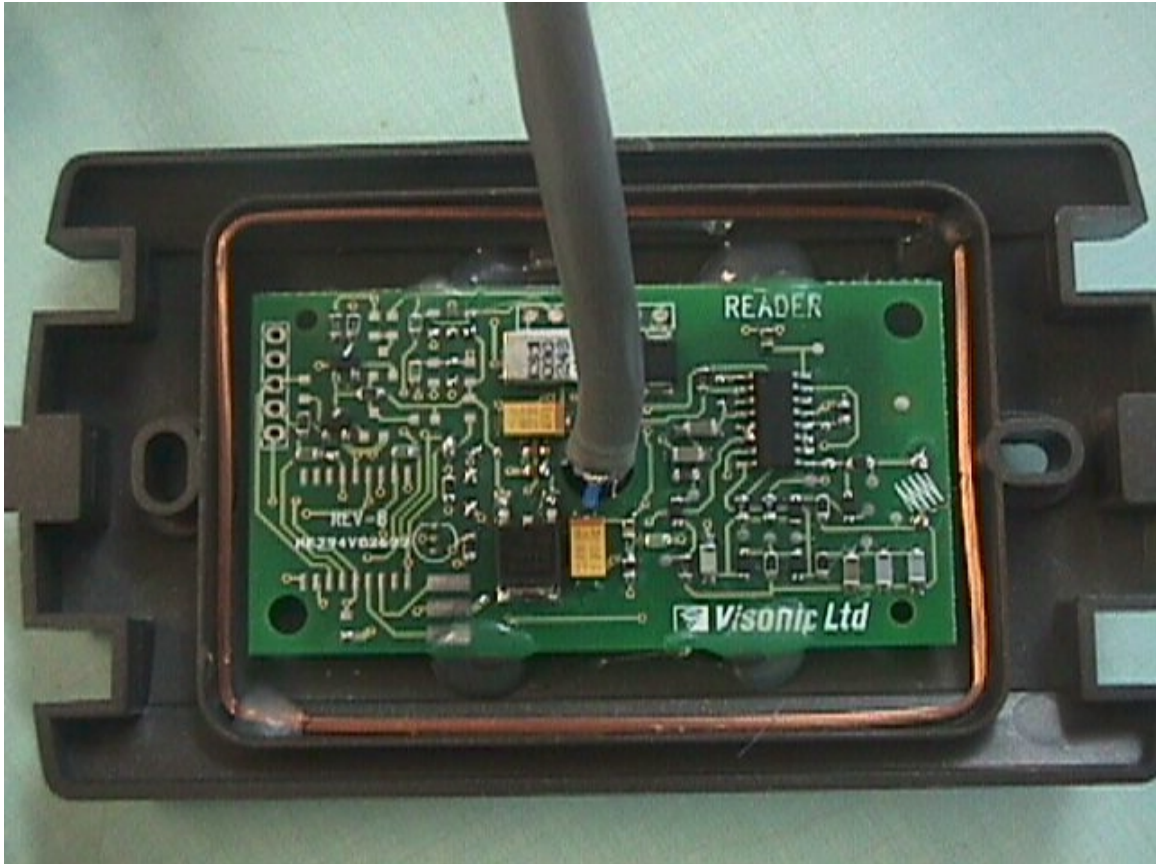
VXS-10 Reader RDR-3, component side
