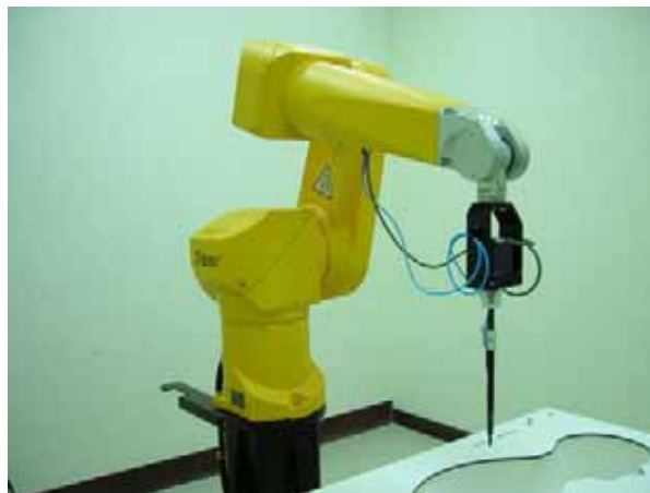
Fig. 5.2 Probe setup on robot
