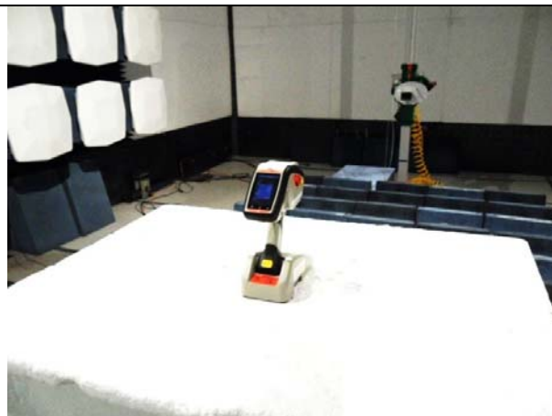
Radiated Emissions (>18GHz) – Rear View
