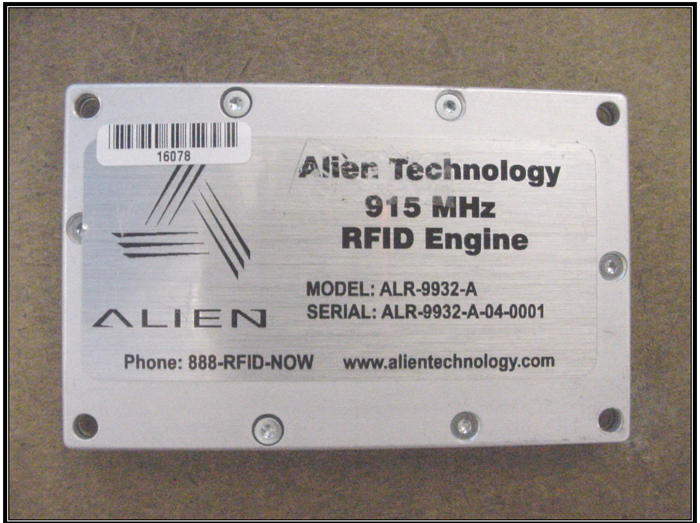
PHOTOGRAPH 8: RFID MODULE FRONT
