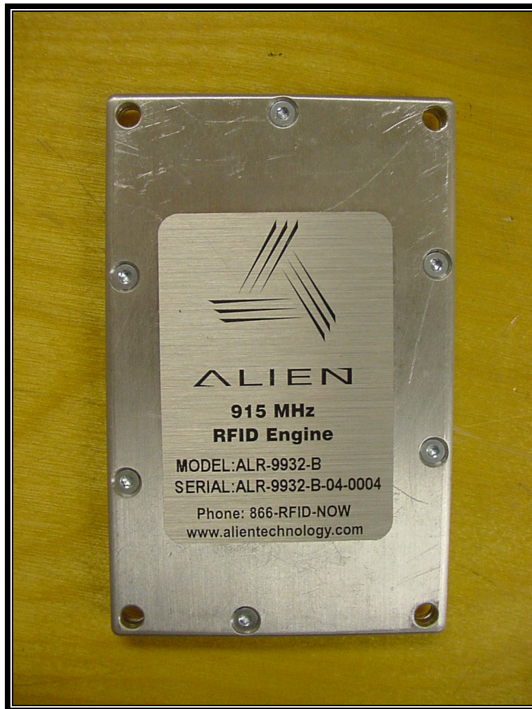
PHOTOGRAPH 8: RFID MODULE FRONT
