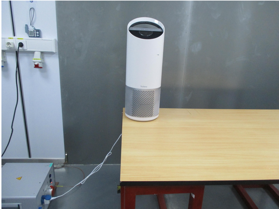
Radiated Emission Test below 1GHz
