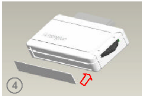
FCC label installed. Attached to assembly with two-sided adhesive film.
