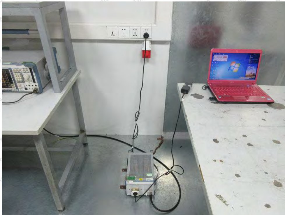
Photo of Conducted Emission Measurement
