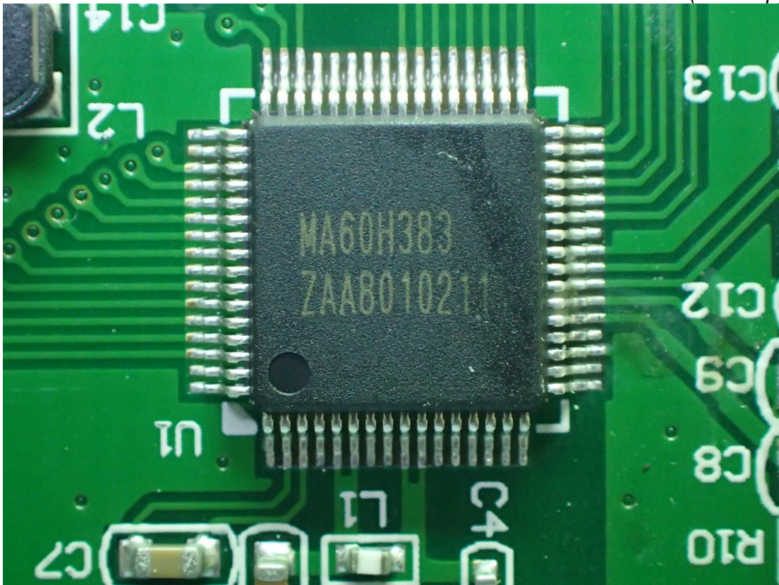
Figure 11 Internal View (RF Chip)
