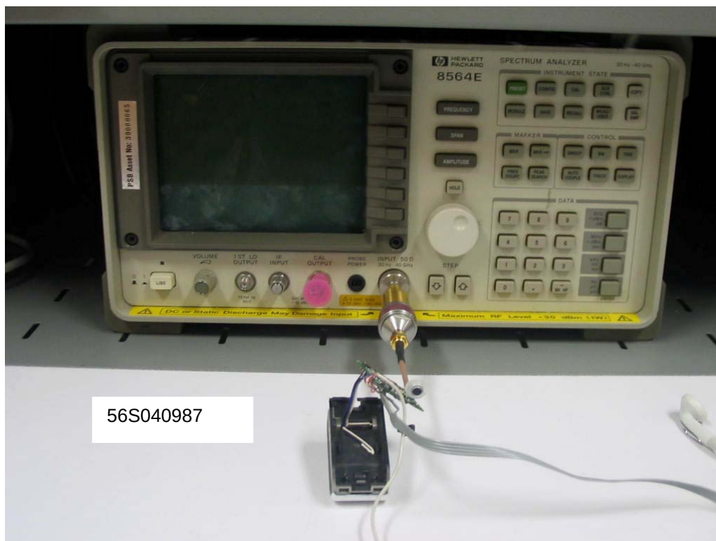
Peak Power Spectral Density Measurement Test Setup
