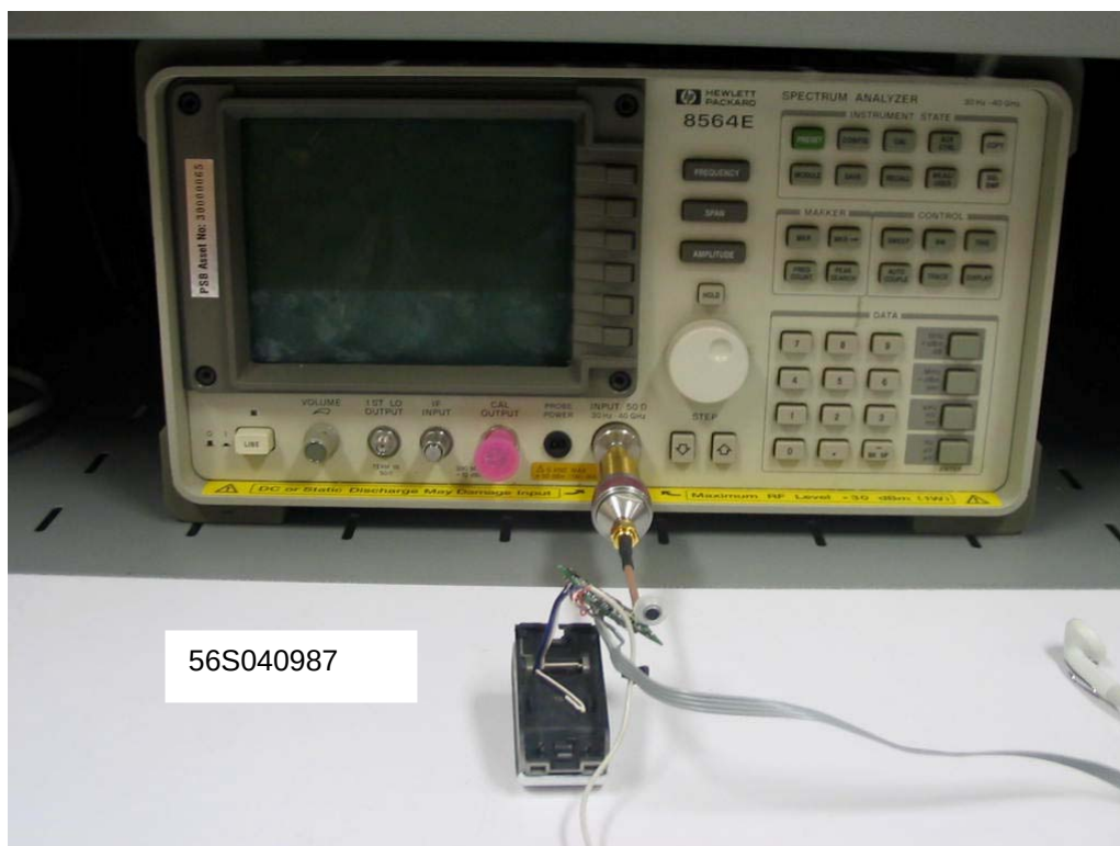
Average Frequency Dwell Time Measurement Test Setup
