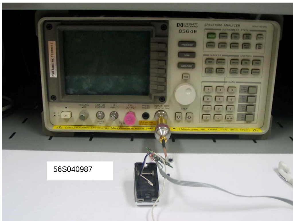
Carrier Frequency Separation Measurement Test Setup
