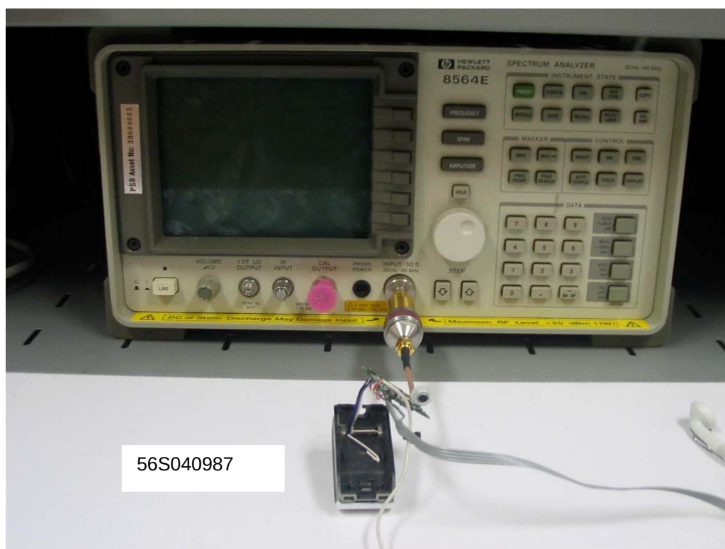
Spectrum Bandwidth Measurement Test Setup
