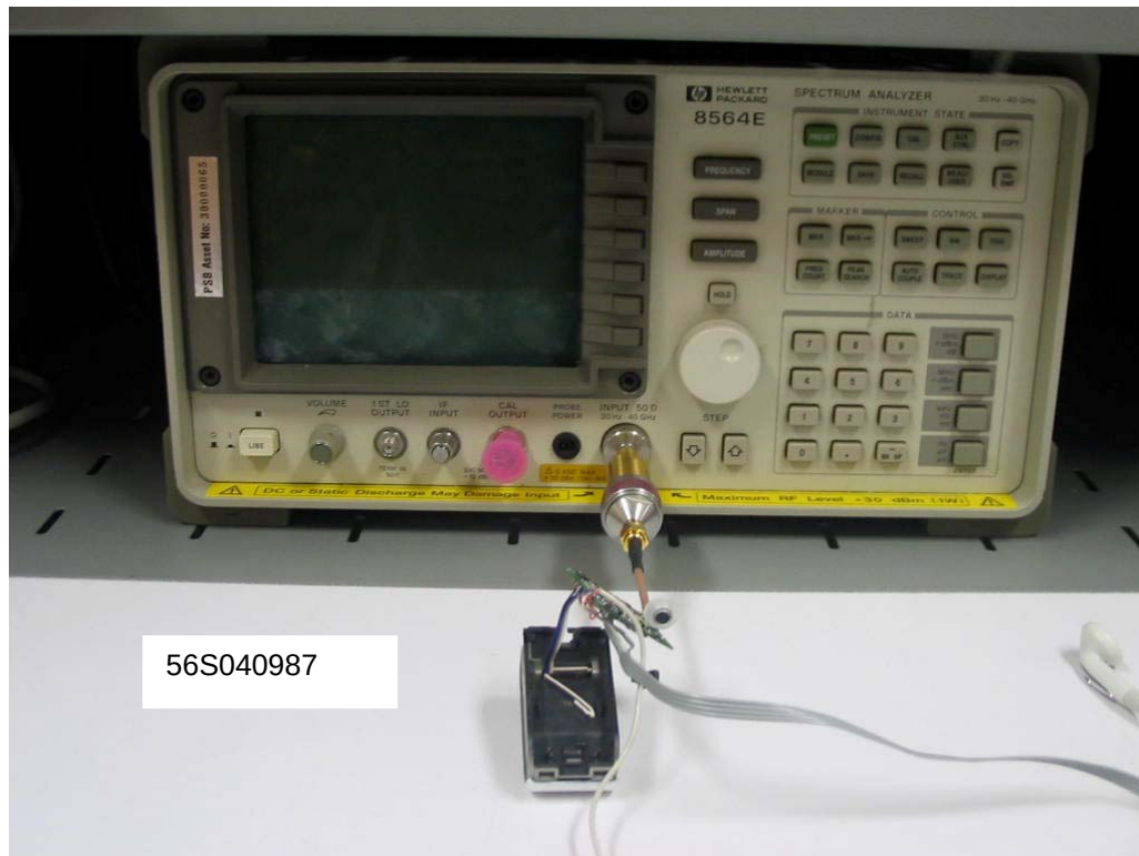
Number of Hopping Frequencies Measurement Test Setup
