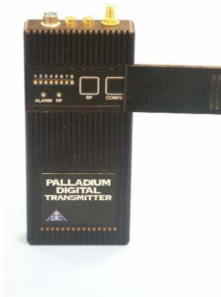
Front With Control Panel Open
