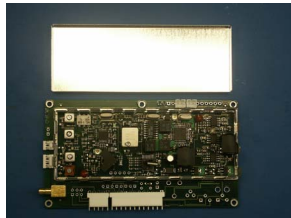
Receiver CCA Top, Shield Off
