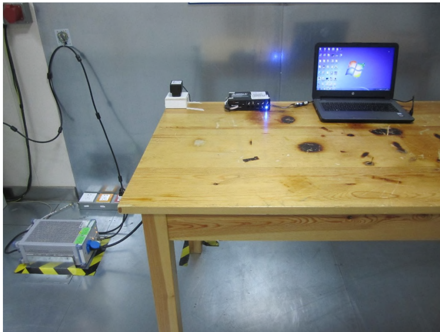
Photograph 3: Set-up for Conducted Emission on AC Mains
