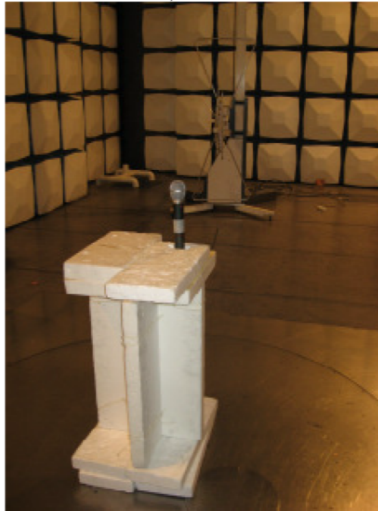
Picture 1: Spurious Radiation Measurement, 30MHz-1GHz
