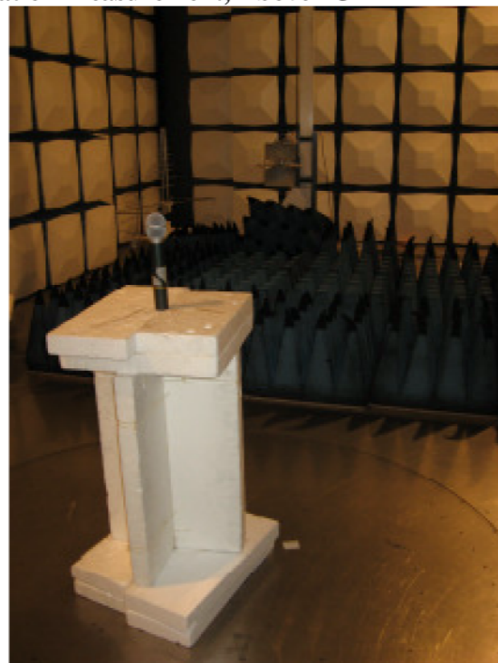
Picture 2: Spurious Radiation Measurement, Above 1GHz
