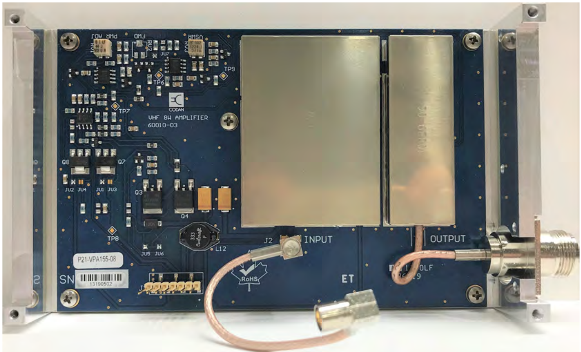
Power Amplifier Board – Top Side, Shields Installed
