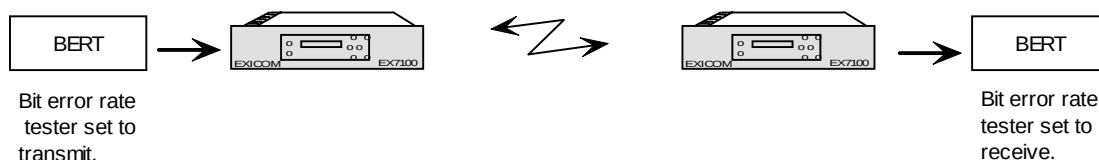
Figure 4.5: End-to-End Bit Error Rate Test
