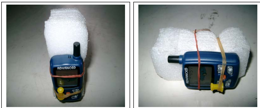
Radiated Open Site Test Set-up (Transmitter Mode)
