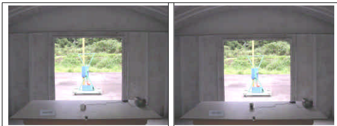
Radiated Open Site Test Set-up
