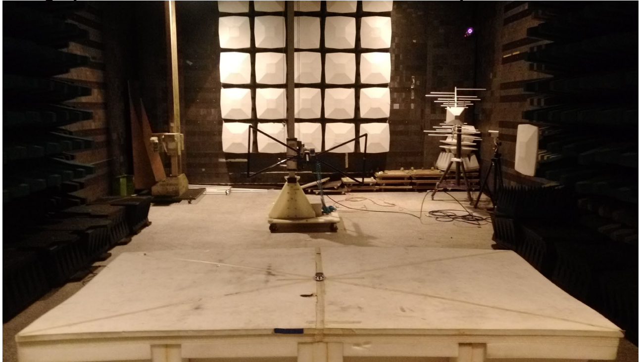
Photograph – Radiated Emission Below 1G Test Setup
