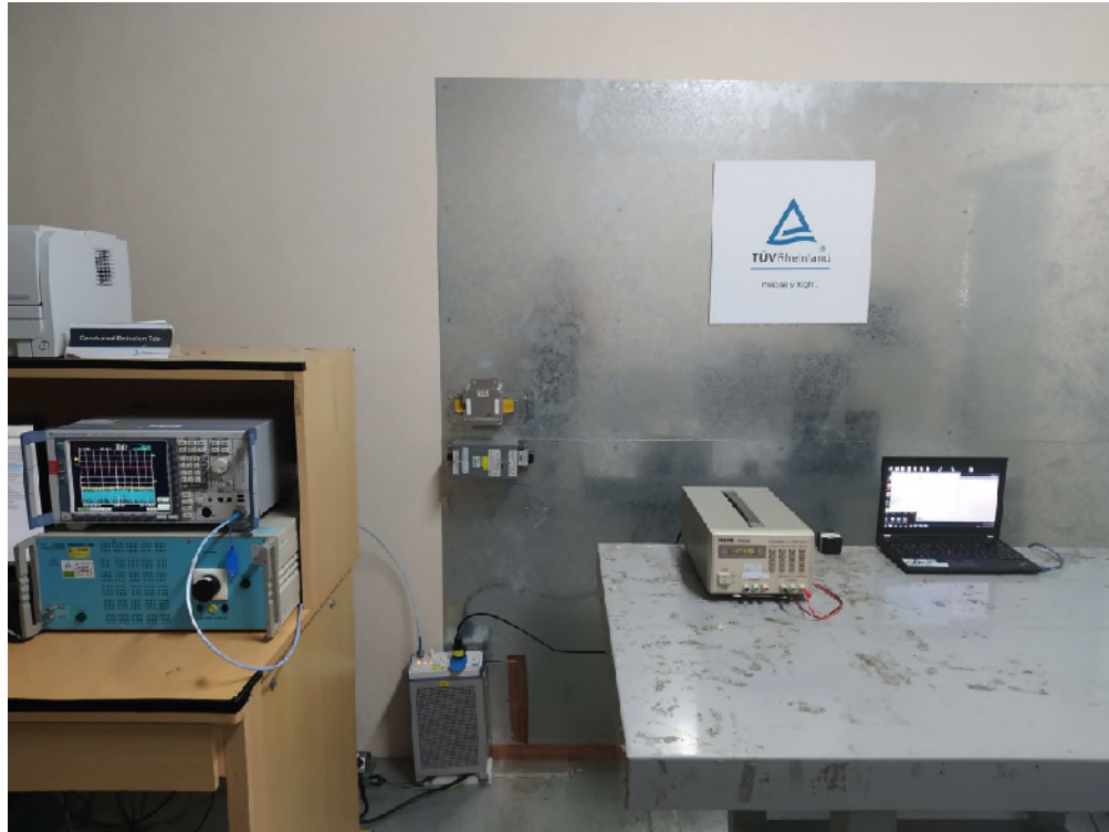
Photograph 7: Set-up for Mains Conducted testing (Front View)
