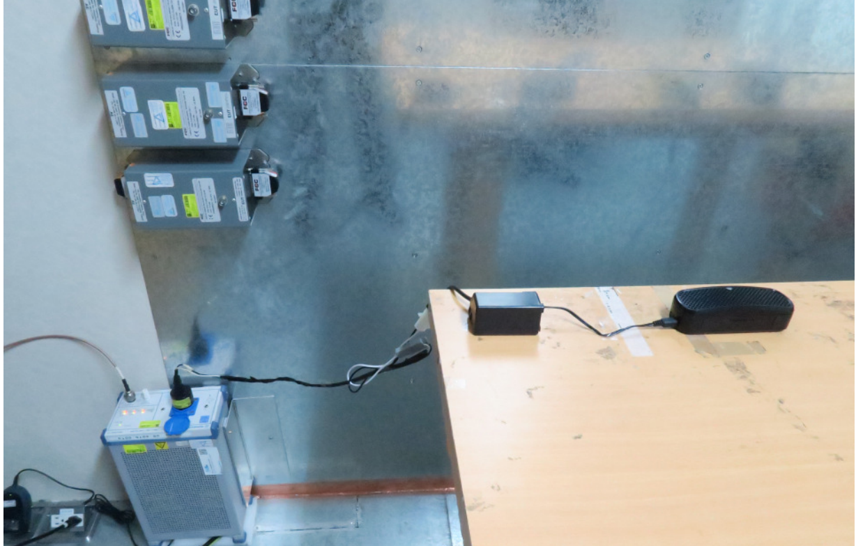
Photograph 6: Set-up for for Mains Conducted testing Front
