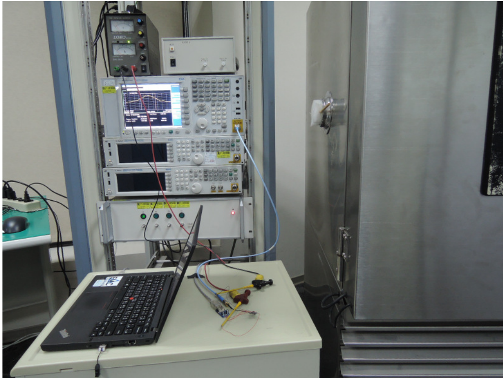
Photograph 4: Set-up for Conducted testing
